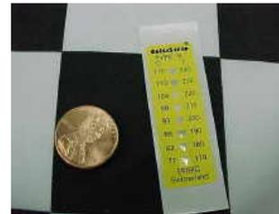
Monitor bearings and other temperature-sensitive parts with these stick-on temperature strips. White heat-sensitive areas are calibrated to specific temperature levels that turn permanently black when exceeded, with an accuracy of  $\pm 1\%$ . Comes in ranges of 170°–240°F (#006-1) and 130°–190°F (#006-2).
