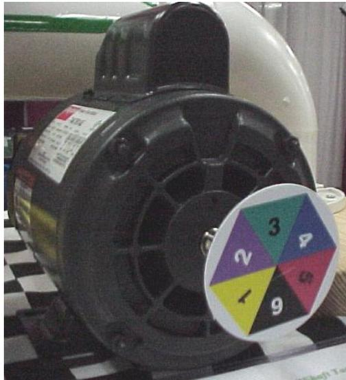
(#024) to the ends of the shafts, rotate a few times, and stop with the next number at the top. Now it's easy to spot the same color on all rotating devices in storage.
